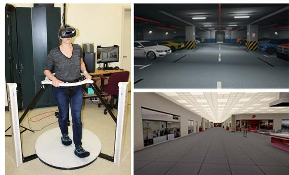
Fig. 1. Left: Virtual reality set-up with the omnidirectional treadmill, VR goggles and hand motion tracker (attached on VR goggles). Right: Examples of VEs (parking lot and corridor in the virtual mall) used for the VR prototype.
