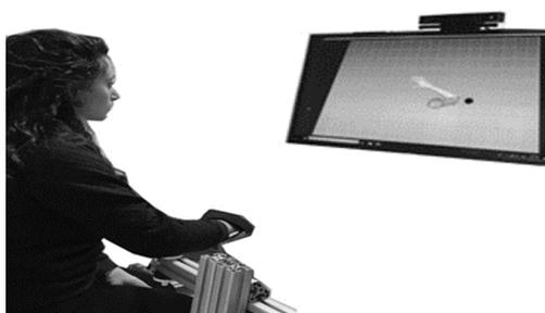
Figure 1: System components: passive manipulator, motion tracking, and VR environment. The presented elbow angle is lower than the actual elbow angle (hypometric).
