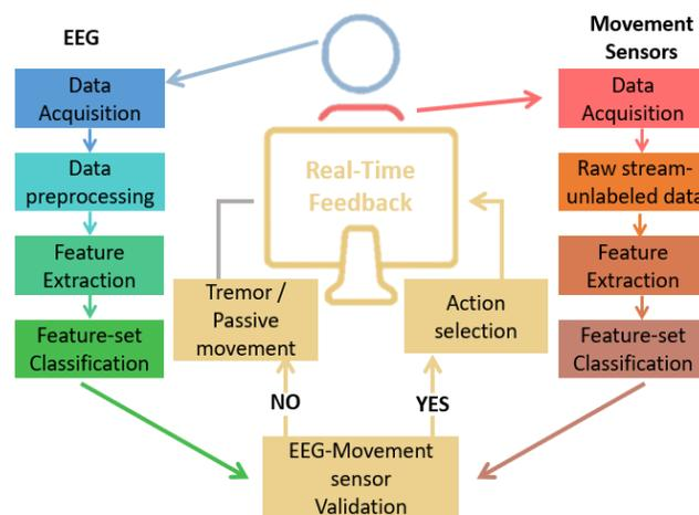
Fig. 1 | A parallel process of data - aquisition, preprocessing, feature extraction and classification that merges to predict user's intention of movement. The two data sources are brain signals recorded with EEG and limb movement as recorded by two small wireless motion sensors worn on the body. The closed loop circuit was shown to possess therapeutic advantages using neurofeedback methods.
