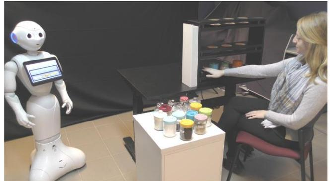
**Figure 1: The experimental set up.** The participant sits facing a height-adjustable table. She has to order the jars on the shelves according to the picture displayed on the robot's tablet. When finished, she has to press the blue button on the bottom-left side of the custom-built shelf unit.
